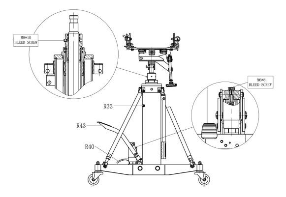
Please follow the instructions to eliminate the air in the pump core if the product is lifting slowly or can't lift up.
